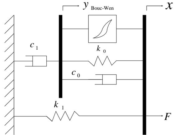
Figure 1. Phenomenological model of MR damper.
